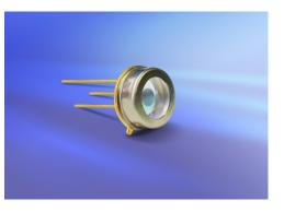
The SXUV5 is housed in a windowless, TO-5 package to allow for responsivity at wavelengths shorter than 150 nm. Other features include shunt resistance of 20 MOhms (minimum) and reverse breakdown voltage of 5 Volts (minimum) to 20 Volts (typical). Capacitance is 500 pF (typical) to 1500 pF (maximum), and response time is from 1 nsec (typical) to 2 nsec (maximum).
